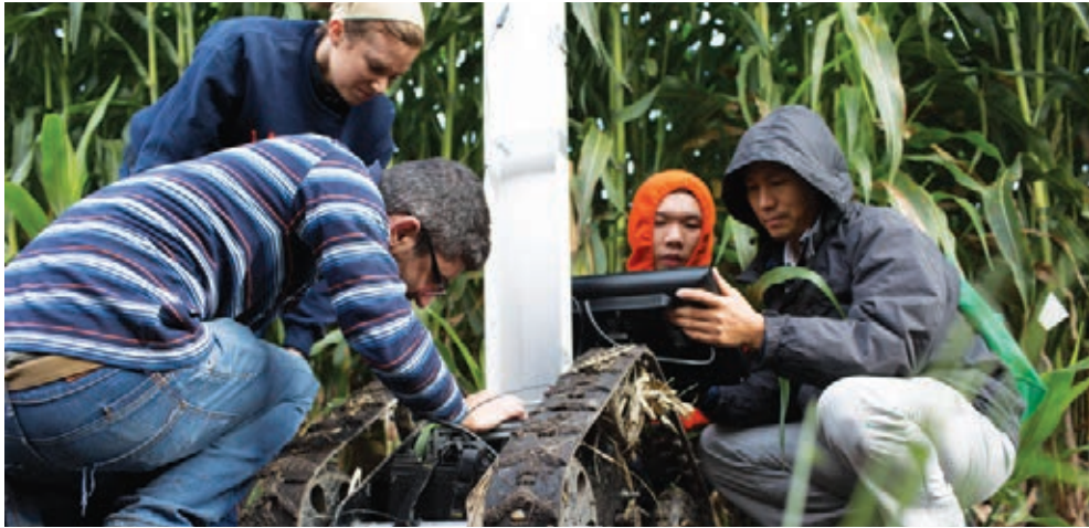
Above: Researchers have developed the TERRA-MEPP robot as a low-cost way to monitor biofuel crops throughout the growing season. The robot treks between rows of crops evaluating the plants on each side simultaneously.
